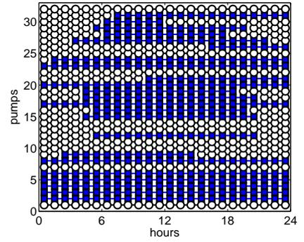
Figure 5b: Active pumps for Test 1
