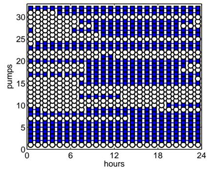
Figure 6b: Active pumps for Test 2
