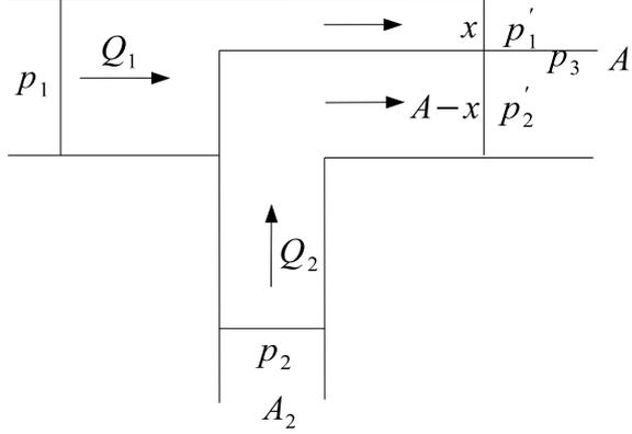
Figure 3: Splitting T-junction into one elbow pipe and one sudden contraction
